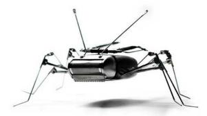
Moving insect is designed using vibration motors
